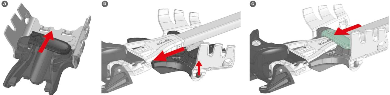
**7** Aktivierung (a, b) – Deaktivierung Harscheisen (c) / Activating (a, b) – Deactivating crampon (c) / Activer (a, b) – Deactiver des couteaux à glace (c) / Attivazione (a, b) – Disattivazione del rampante (c) / Activando (a, b) – Desactivando la cuchilla (c)
